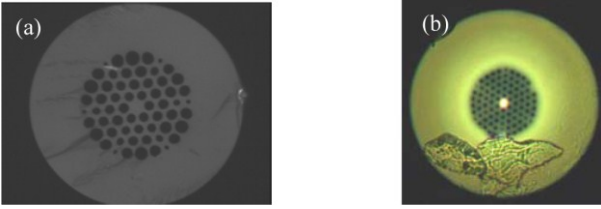
Figure 6. (a) Cross section images of (a) pure-silica PCF (IPHT-84b1a) and Ge-doped PCF (IPHT-282b5).
