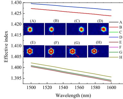
Fig. 2. Simulation of the first eight mode fields and their dispersion curves of the partially filled D-C PCF; inset: (A-B) the mode profiles of the  $\text{LP}_{01}$  of core *a*, (C-D) the mode profiles of the  $\text{LP}_{01}$  mode of core *b*, and (E-H) the mode profiles of the  $\text{LP}_{11}$  mode of core *a*.
