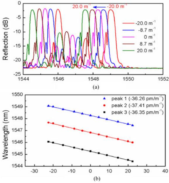
Fig. 9. Bend response of the TC-FM FBG with different bend curvature in the bend direction of  $\theta$  equals  $0^\circ$ . (a) Reflection spectra evolution of the TC-FM FBG with different bend curvature. (b) Wavelength shift of the three resonance peaks in the reflection spectra of the TC-FM FBG as a function of bend curvature.
