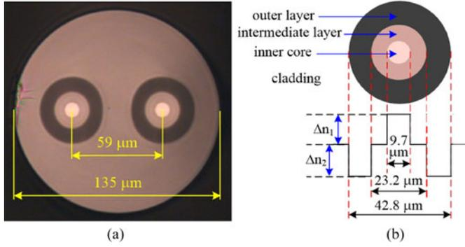
Fig. 1. Schematics of the twin-core few-mode fiber (TC-FMF). (a) Microscopic image of the cross-section of the TC-FMF. (b) Refractive index profiles of one fiber core of the TC-FMF.
