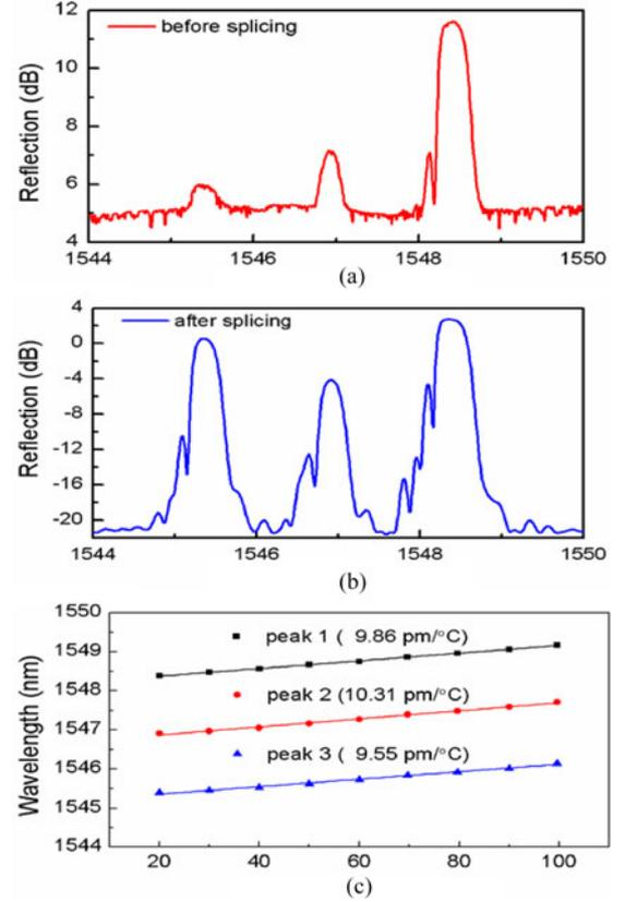
Fig. 5. (a) Reflection spectrum of the TC-FM FBG before splicing. (b) Reflection spectrum of the TC-FM FBG after splicing. (c) Wavelength shifts of the three reflective resonance peaks of the TC-FM FBG as a function of ambient temperature.
