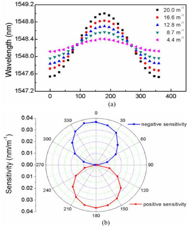
Fig. 8. (a) Resonant wavelength of peak 1 in the reflection spectrum of TC-FM FBG as a function of the bend direction angle  $\theta$  under different bend curvatures. (b) Bend sensitivities of the TC-FM FBG in different bend directions ( $\theta$ : from  $0^\circ$  to  $360^\circ$ ).
