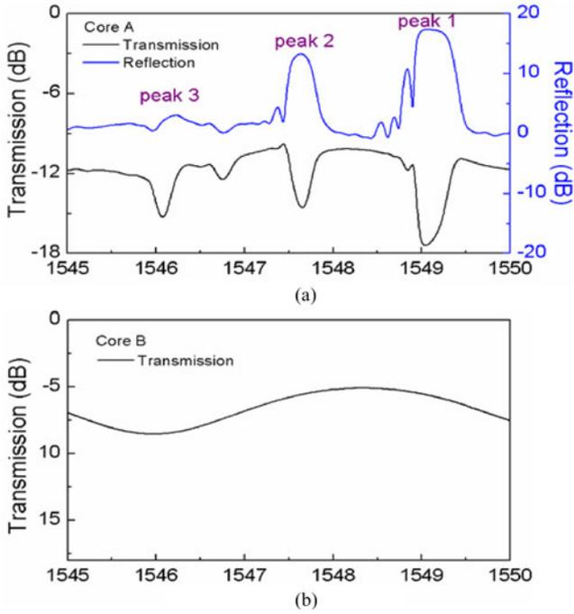
Fig. 3. Optical spectra of the TC-FM FBG. (a) Transmission and reflection spectra in core A of the TC-FMF. (b) Transmission spectrum in core B of the TC-FMF.
