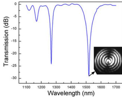
Fig. 1. Experimentally measured transmission spectrum of LPFG with grating pitch of  $450 \mu\text{m}$ . Inset: measured near mode field at resonance dip  $1518.7 \text{ nm}$ .
