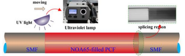
Fig. 2. Schematic of the NOA65-filled PCF. The insets side image shows the fusion joint of the NOA65-filled PCF with a single mode fiber.
