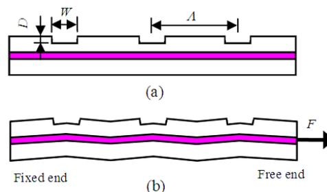
Fig. 4 Schematic diagram of the CO<sub>2</sub>-laser-induced LPFG with asymmetric grooves (a) before and (b) after a stretching force is applied to the grating.
