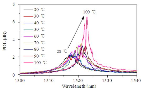
Fig. 6 Polarization dependence evolution of the CO<sub>2</sub>-laser-induced LPFG with the rise of temperature.
