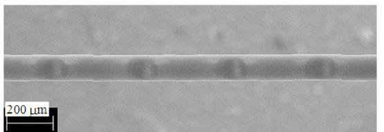
Fig. 1 SEM image of the asymmetric CO<sub>2</sub>-laser-induced LPFG with periodic grooves (grating pitch: 400 m; number of periods: 20).
