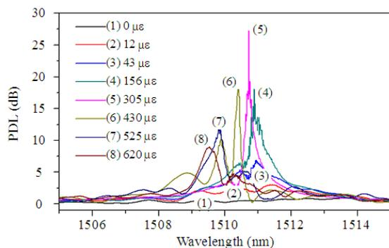
Fig. 3 Polarization dependence evolution of the CO<sub>2</sub>-laser-induced LPFG with an increase in the tensile strain applied.
