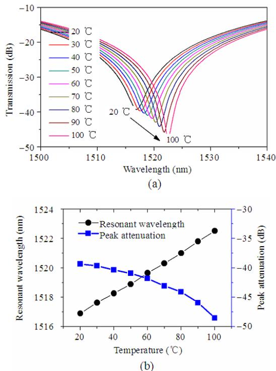
Fig. 5 Temperature response of the CO<sub>2</sub>-laser-induced LPFG: (a) transmission spectrum evolution of the CO<sub>2</sub>-laser-induced LPFG with the rise of temperature and (b) resonant wavelength and peak attenuation of the LPFG as a function of temperature.
