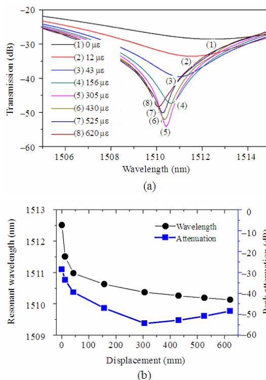
Fig. 2 Strain response of the CO<sub>2</sub>-laser-induced LPFG: (a) transmission spectrum evolution of the CO<sub>2</sub>-laser-induced LPFG with an increase of the tensile strain applied, and (b) resonant wavelength and peak attenuation of the LPFG as a function of the tensile strain.
